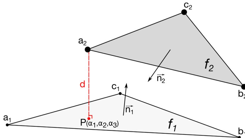
**Figure 4-2.** Contact detection conditions between two faces.
