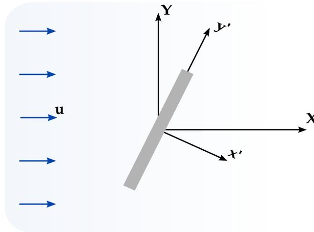
**Figure 5-3.** Anisotropic porous media vectors definition (PMMID = 4). The vectors  $\mathbf{X}$  and  $\mathbf{Y}$  are the global axes;  $\mathbf{x}'$  and  $\mathbf{y}'$  define system for the primed coordinate  $(x', y', z')$ .
