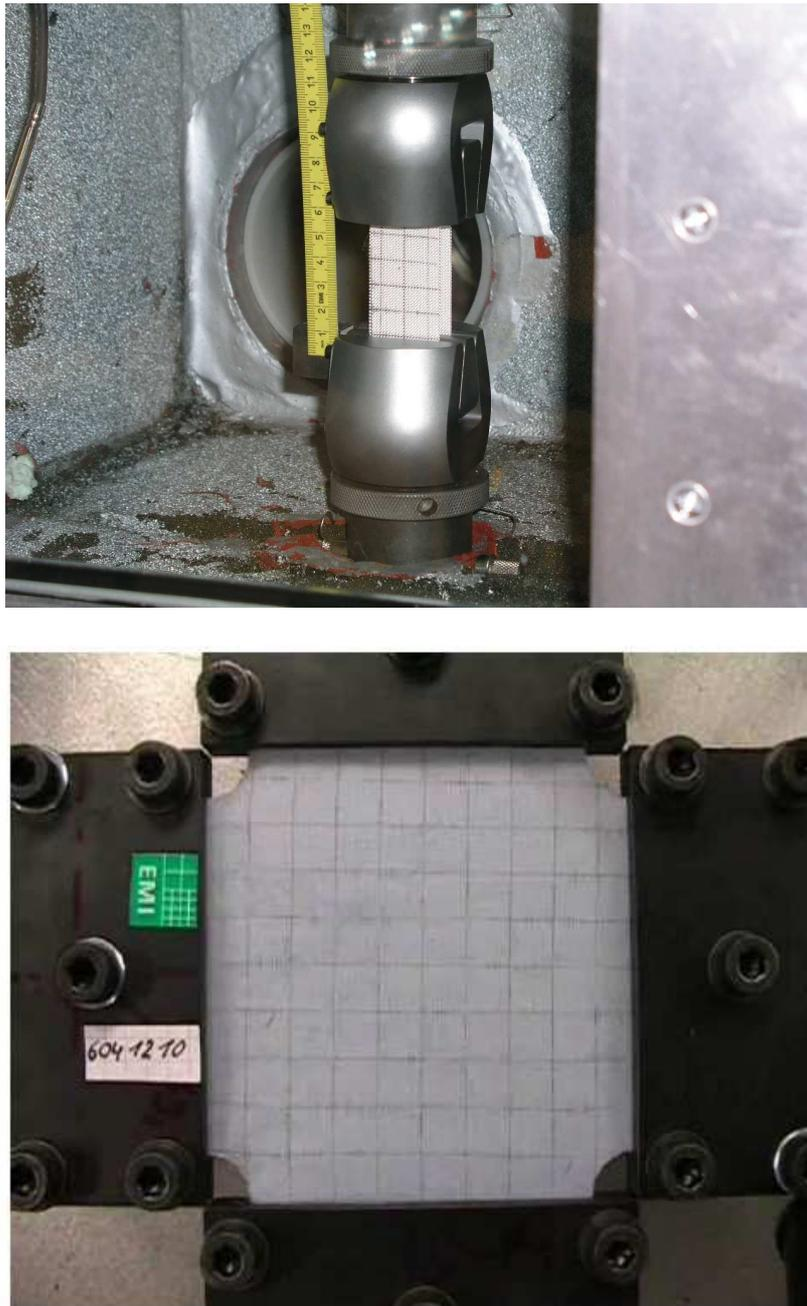
Figure 1 Uniaxial (top) and biaxial (bottom) test setup.
