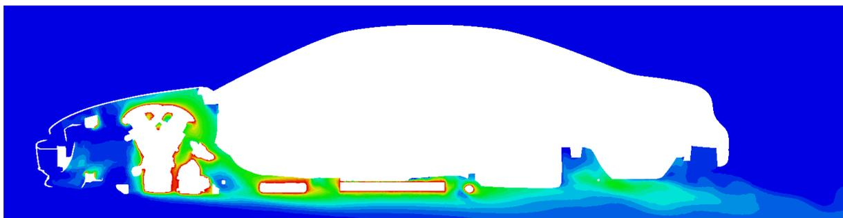
Figure 9: fluid temperature in a cutplane at the symmetry plane.
