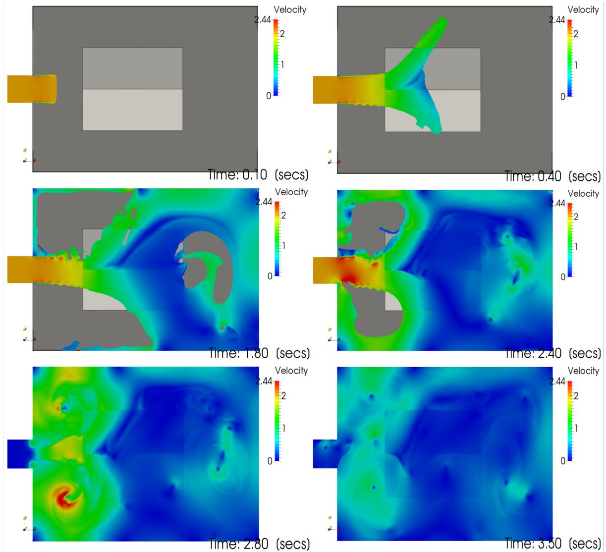
Figure 7: RTM sequence in multi-porous domain.
