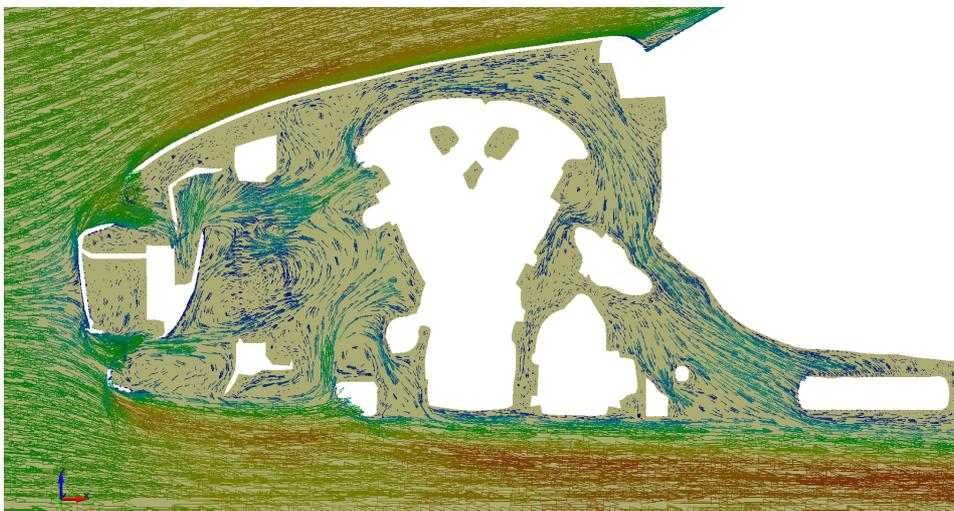
Figure 12: Flow field inside the engine compartment and the radiator.
