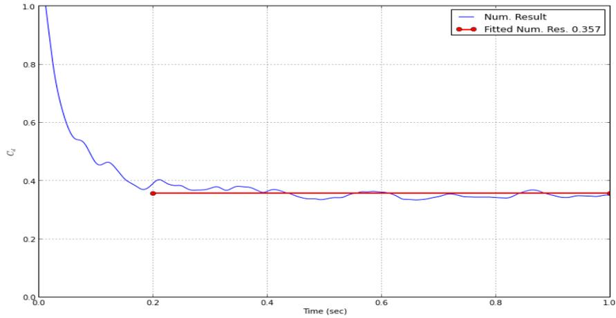
Figure 10: Drag force without the radiator.
