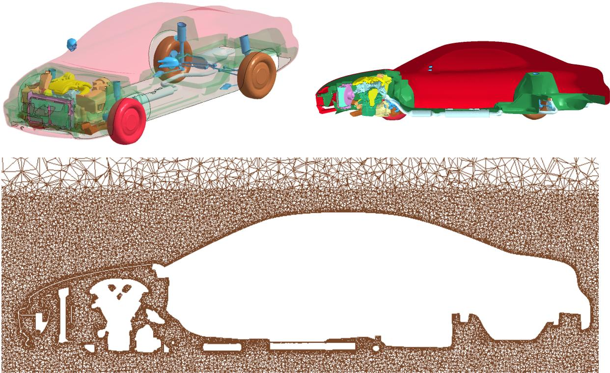
Figure 8: Geometry and volume mesh of a GM Pontiac model.
