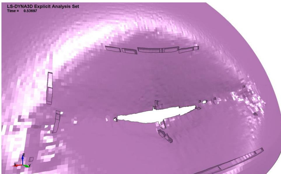
Fig.13: Perforation of the dome from the analysis with SPH model
