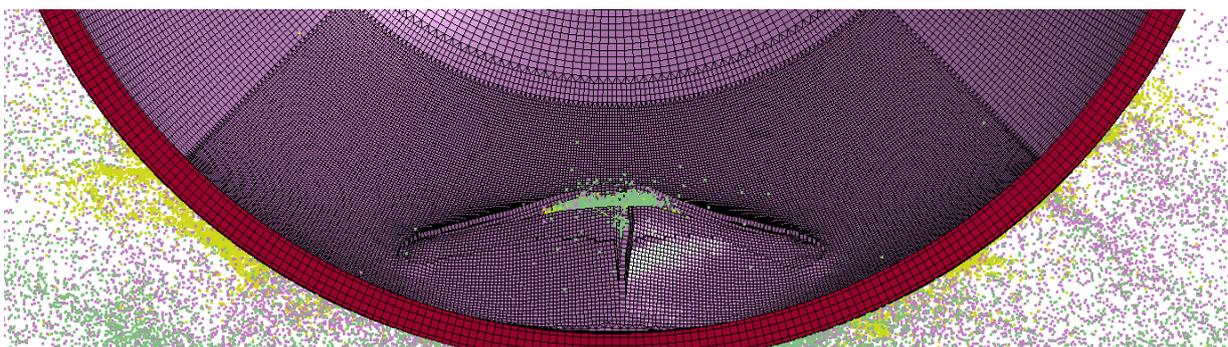
Fig. 15: Penetrating SPH into the containment structure, bottom-up view
