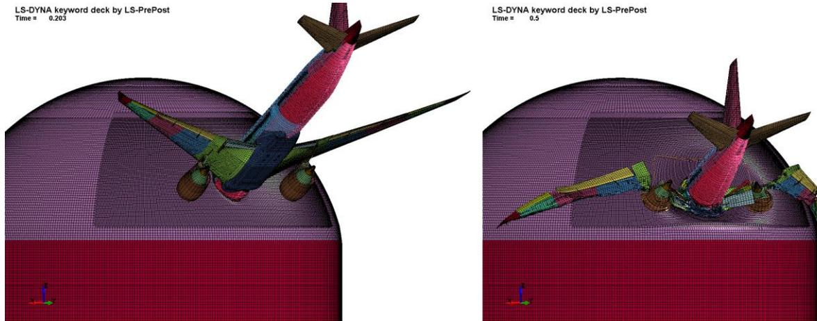
Fig.5: Impact at the containment with “rigid mass” model
