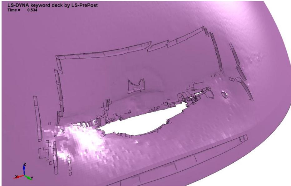
Fig.12: Perforation of the dome from the analysis with “rigid mass” model
