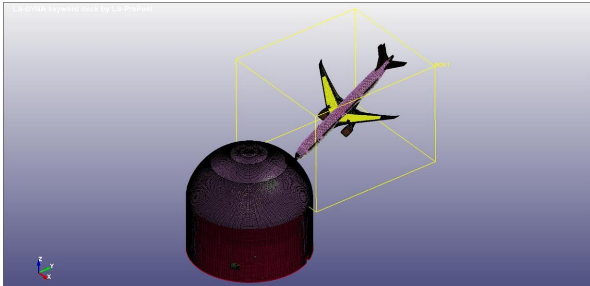
Fig.4: Box for the SPH approximation
