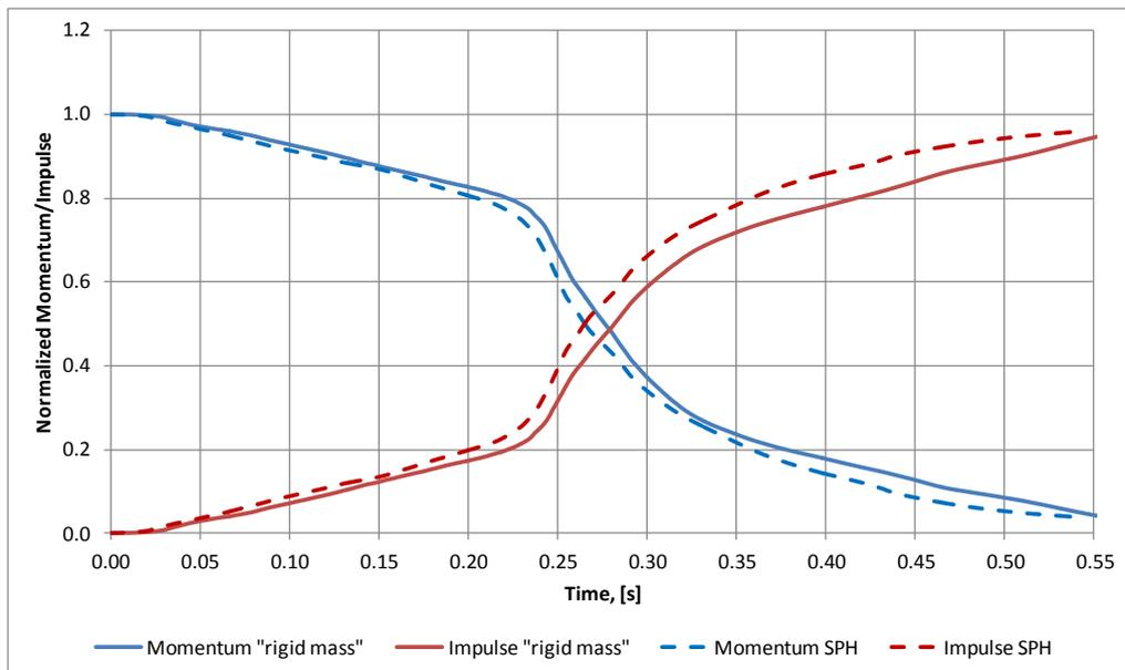
Fig.10: Normalized momentum and impulse of the contact force of the considered analyses
