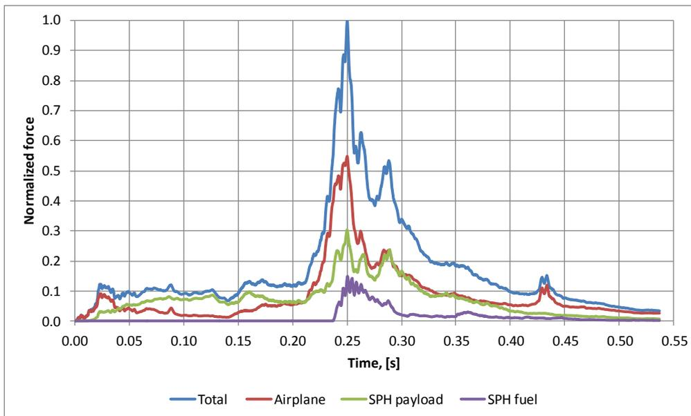
Fig.8: Resultant contact force from the analysis with SPH model of the non-structural mass
