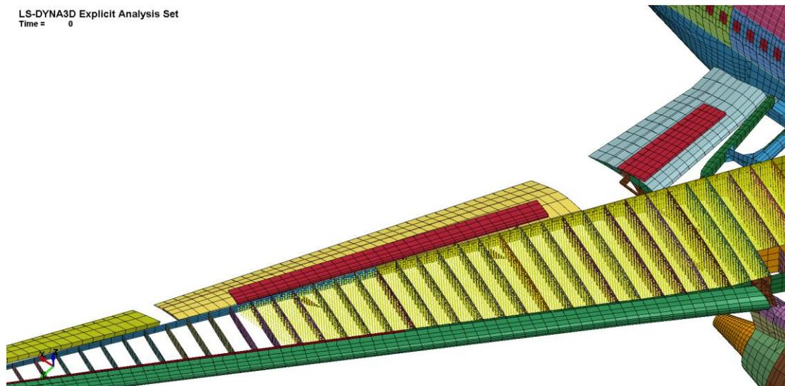
Fig.3: SPH fuel particles
