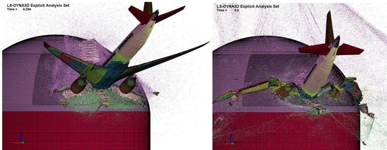
Fig.6: Impact at the concrete containment with SPH model
