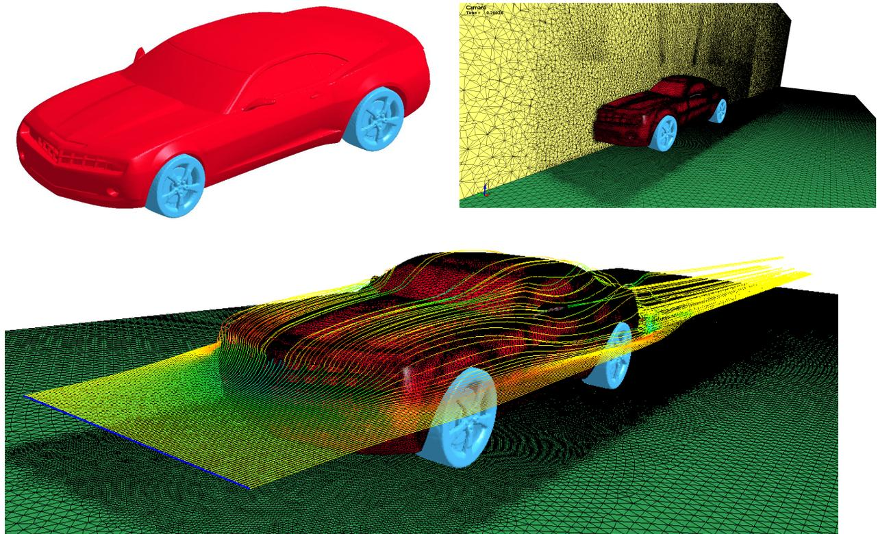
Fig.4: CFD analysis of a vehicle which will be used for FSI simulation.
