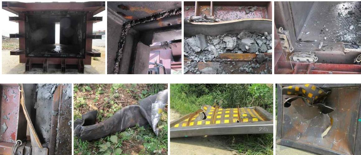
Fig. 10: Damage configurations of partial chamber bulkhead under internal blast test with 2xHE TNT at  $1/16L$  stand-off distance
