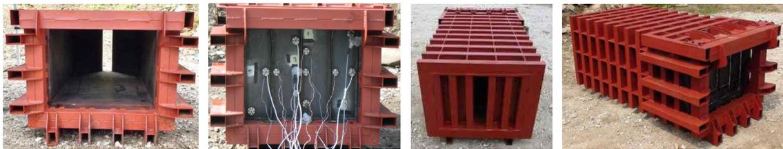
(a) front view without bulkhead (b) front view with bulkhead (c) rear view with opening (d) iso view of chamber test model
