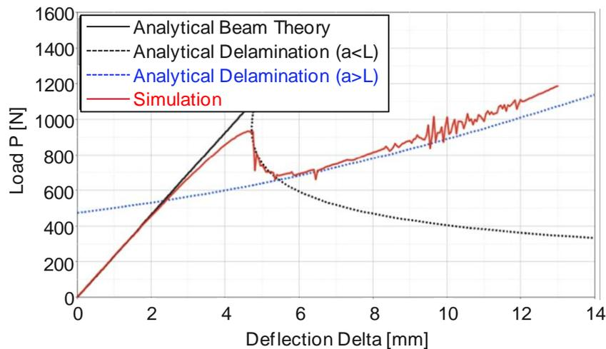
Fig.16: Simulation result of ENF test of CFRP with an element of 3.0 mm
