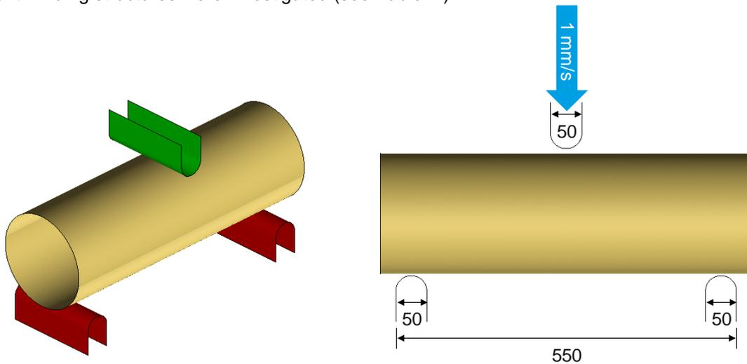
Fig.8: 3PB test
