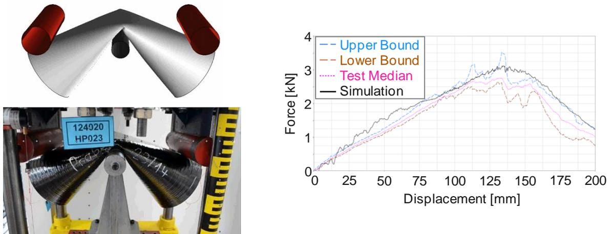
Fig.11: Comparison of test and simulation of 3PB on tubular CFRP specimen with set-up type 2
