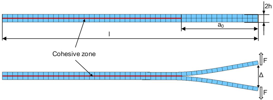
Fig.12: FE model of DCB test specimen in undeformed (top) and deformed (bottom) shape
