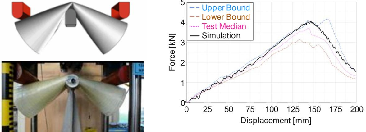
Fig.10: Comparison of test and simulation of 3PB on tubular GFRP specimen with set-up type 2
