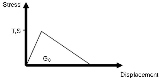
Fig.6: Bi-linear traction separation law for pure mode [13]
