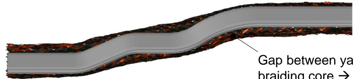
Gap between yarn and braiding core → matrix-rich zones
