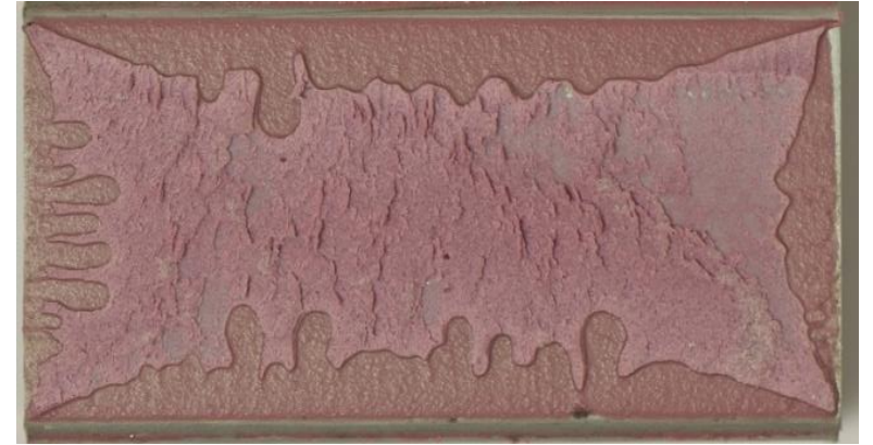
Viscous fingering on a LWF KS2-Specimen
