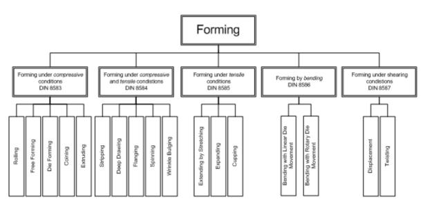
Figure 1: Subdivision of manufacturing processes according to DIN 8582
