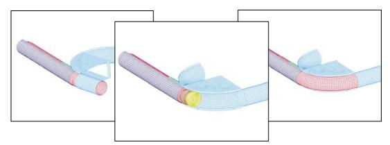
Figure 2: Process-Chain of the hydroforming showing bending, preforming and hydroforming
