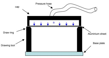
Figure 4: The concept of the experimental tool for the warm metal forming process
