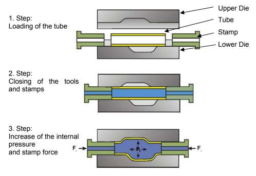
Figure 3: Operation sequence of the hydroforming process of a tube
