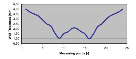
Figure 6: Diagram showing the absolute values of the measured wall thickness distribution of a formed part
