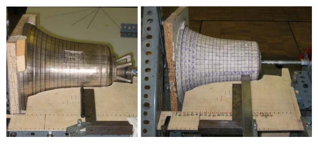
*Figure 1.* Customized measure construction, left: capture of the outer surface of the bell, right: capture of the inner surface via the plaster cast
