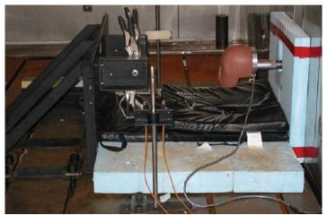
Figure 7: Free Motion Head form test set-up.
