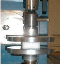
Figure 3a: Quasi-static compression test.
