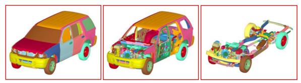
Figure 2: Finite Element Model of the Exemplar Vehicle
