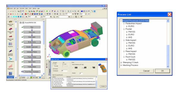
Fig. 6: Visual-Process and Process Templates of regulatory test procedures
