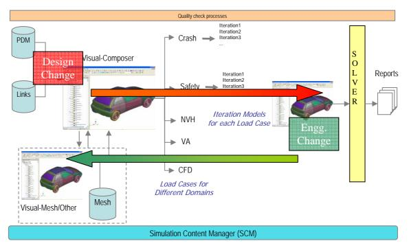
Fig. 9: Propagation of Design and Engineering Change
