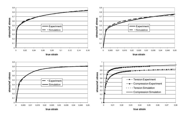
Fig. 2: Comparison of experimental and numerical results. Upper left: uniaxial tension in RD. Upper right: uniaxial compression in RD. Lower left: uniaxial compression in RD after 10% tensile pre-strain in RD. Lower right: uniaxial tension and compression in TD, respectively, after 10% tensile pre-strain in RD.
