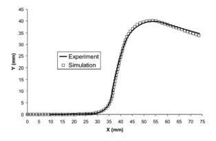
Fig.3: Comparison of experimental and numerical results: released sheet strips after drawing (the half of the geometry is displaced).
