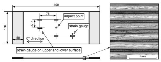
Fig. 1: Dimensions of impact test specimens (in mm) and micrograph of composite laminate
