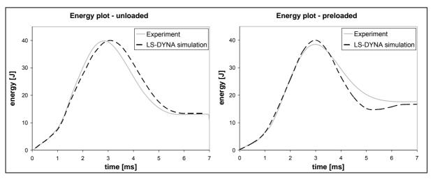
Fig. 6: Energy plot in experiment and simulation for unloaded and preloaded plates
