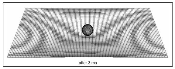
Fig. 4: Reference model for low velocity impact simulations on preloaded composite plate
