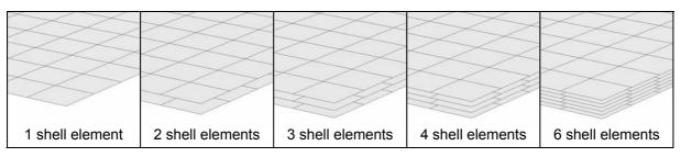
Fig. 11: Overview of different number of shell element layers for the composite laminate modelling
