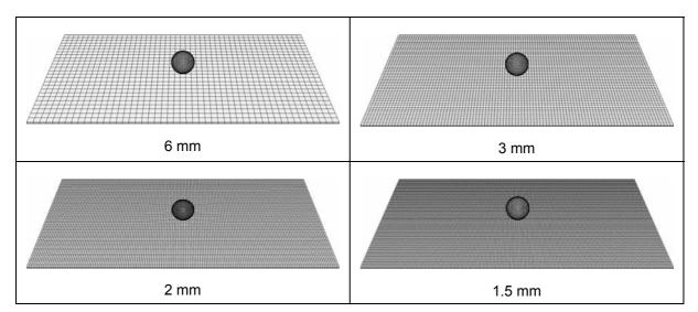
Fig. 9: Overview of different mesh sizes for composite plate with element lengths from 1.5 to 6 mm
