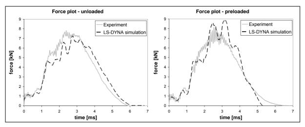
Fig. 5: Contact force plot in experiment and simulation for unloaded and preloaded plates
