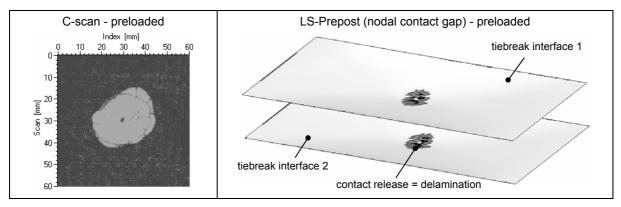
Fig. 7: Extent of delamination in experiment and simulation for preloaded plate
