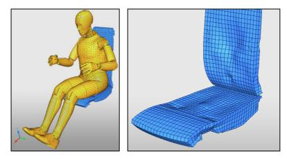
Fig. 15: Result of the deformed seat using the seat deformer.
