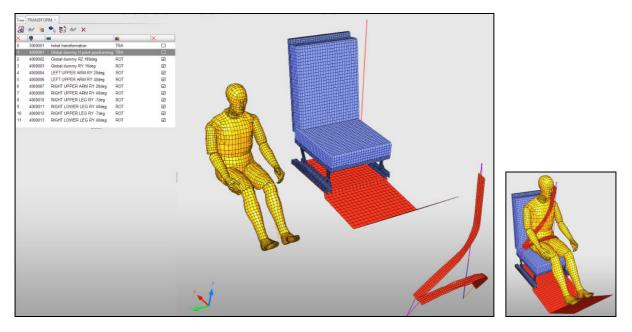
*Fig. 4: The transformation manager provides a list of available transformations in the model. The positioning of the dummy and the belt system is deactivated in the left screenshot.*
