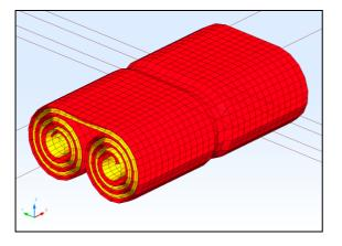
Fig. 16: Result of a folded and rolled circular airbag after automatic mesh generation.
