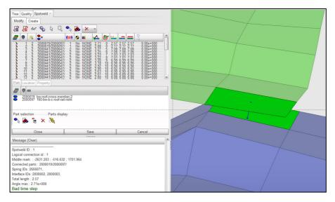
Fig. 8: Connector information can be imported from file. Connected parts, location of the spotweld and properties can be checked/modified in the Spotweld Browser.
