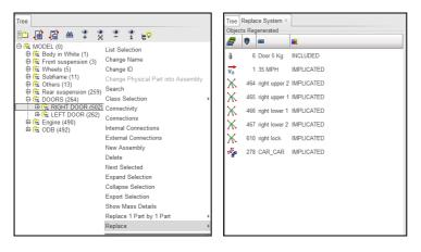
Fig. 5: In the replace system window, the list of the features rebuilt by HyperCrash is displayed.
