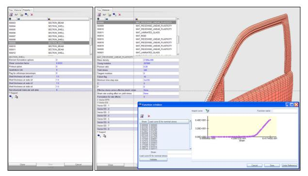
Fig. 10: Property and material browsers with separate function window for curve review.
