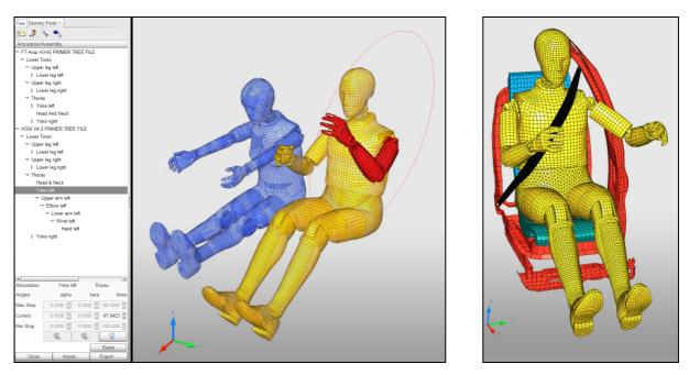
Fig. 14: Dummy positioning tool and seatbelt generator. The example shows the positioning of two Hybrid III 5% and 50% dummies with tree view in parallel.
