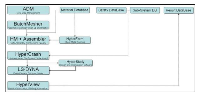
Fig. 1: Positioning and use of HyperCrash in the Altair HyperWorks environment.
