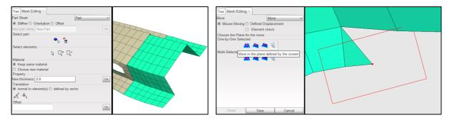
Fig. 9: Example of useful mesh editing tools, part stiffeners can be created automatically and nodes can be moved in plane defined by the screen.
