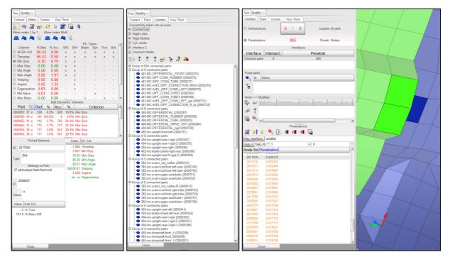
Fig. 7: Examples for element quality check, part connection check and intersection/penetration check.
