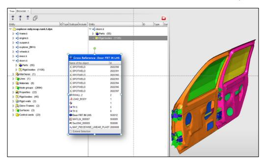
Fig. 3: Model Browser with include file management and cross-reference viewer display. The list shows material and property of part "Door FRT IN LHS" (bold) as well as all entities (spotwelds, time history sets, contact definition, rigid wall, gravity load) that have a reference to this part.
