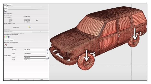
Fig. 13: Automatic mass balance with prescribed weight on the front/rear tires.
