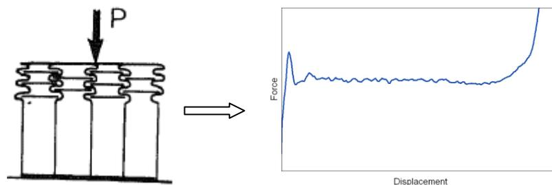
Figure 2: Buckling and force-deflection behaviour of T-directional loaded honeycomb structure [3]
