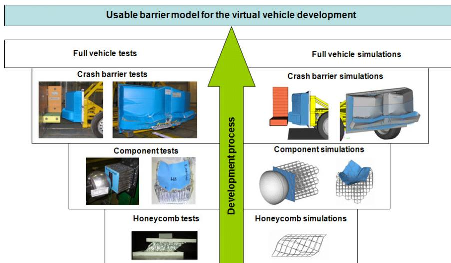
Figure 9: Development process of IHS crash barrier model based on DBM
