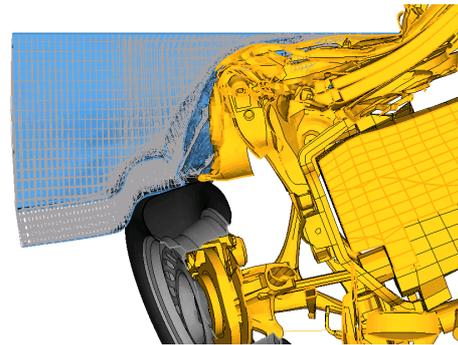
Figure 22: Vertical cut of ODB and front end
