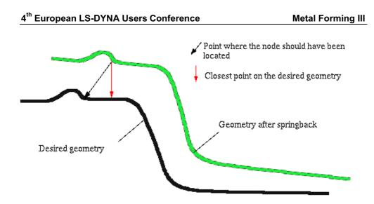
Figure 1 Problem with measuring deviation between different geometries
