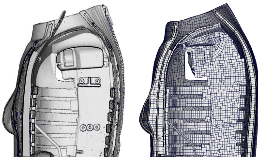
(a) CT Scan Data (b) FE Model Figure 3: Comparison of Thorax Section
