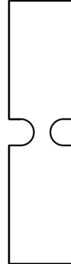
R4 notched tensile test R4Fz
