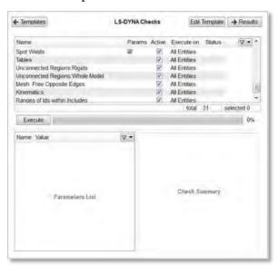
The Checks Manager presents the results of the checks color-coded in groups of per type error based on the category of the error or warning. Tools are provided to automatically fix errors from within the Checks Manager interface.
