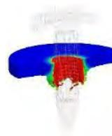
Flow drill screwing (FDS)
