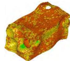
RVE for nano-particle reinforced rubber
