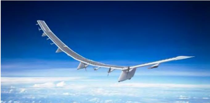
*Hawk30 solar-powered high-altitude platform system will serve as a stratospheric telecommunications platform for delivering next-generation global connectivity.*
