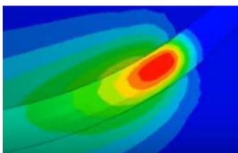
[\*\*Thermal part of welding simplest simulation in LS-DYNA\*\*](#)
