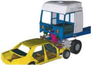
Impact of a passenger car (W124) with 60 km/h relative velocity. Source: DaimlerChrysler AG
