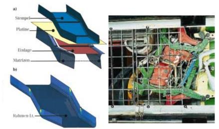
Perpendicular impact onto a rigid barrier at 50 km/h with 40% coverage (left: FEM simulation, right: Test)
