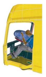
Actros passenger simulation (with **belt and belt-tightener**) for optimal airbag passenger protection. Source: DaimlerChrysler AG
