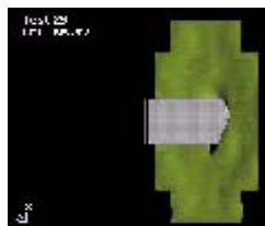
Test 29 4 plies Zylon Gripped on 4 edges 96 g fragment
