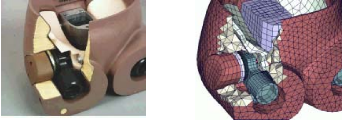
Figure 9: Parts interacting in pelvis area, dummy and finite element model.
