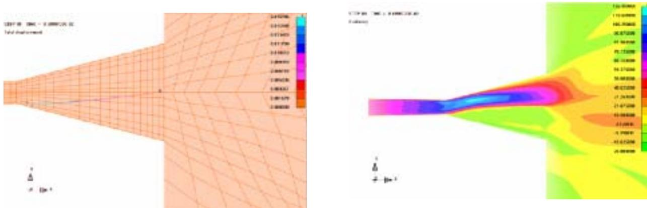
algorithm (Monotone Upwind Schemes for Conservation Laws). The fluid was modeled using LS-DYNA constitutive model #9 with a linear polynomial equation of state. The mobile longitudinal partition was modeled using a linear elastic constitutive law.
