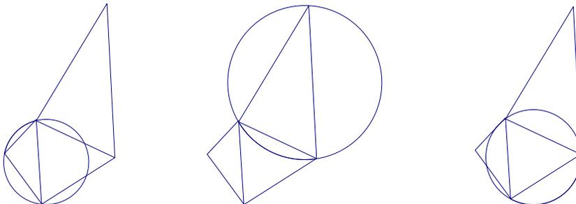
The Delaunay method is used to produce a Delaunay mesh for an arbitrary set of points in the plane. In fact, such triangulations are unique under reasonable restrictions on the points.
