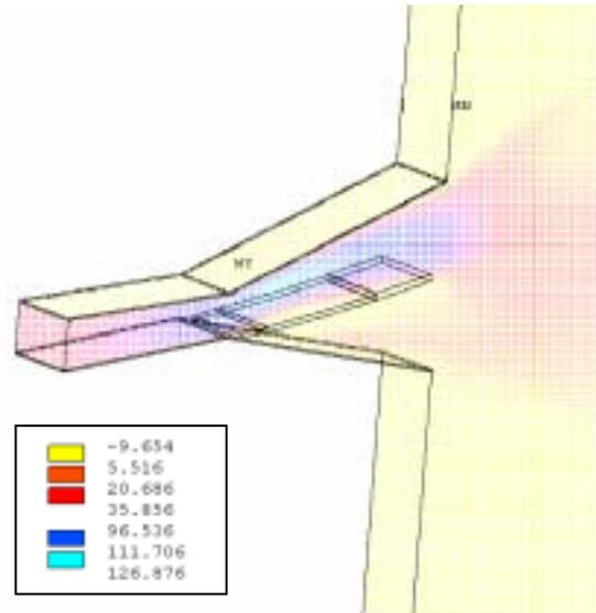
The numerical investigation of the GPJ-process in LS-DYNA was carried out with use of ALE-technology (Arbitrary Lagrangian-Eulerian formulation) jointly with the Van Leer MUSCL
