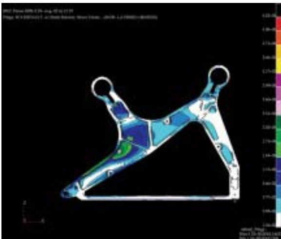
Nastran Stress Plot of Seat Bracket
