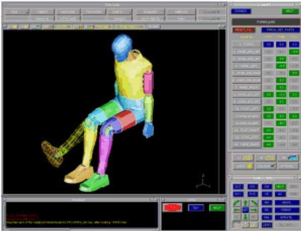
Dummy positioning facility that detects stop angles and rotational degrees of freedom
