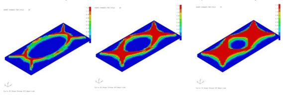
2. Distortion Constraints. This new feature automatically creates distortion constraints that can dramatically reduce distortion that can occur in shape, topography and freeform optimization.
