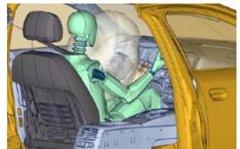
Optimization of Restraint Systems with LS-OPT at Audi.
