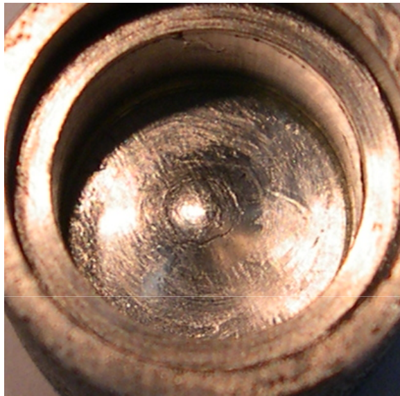
circumferential crack at bottom side
