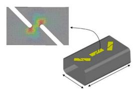
absorption under crash loadings. However, such materials exhibit a highly orthotropic behavior both in plasticity and in failure for which an orientationdependent damage accumulation is necessary for accurate results. Polymers are a further example of materials that, under certain circumstances, require a more advanced treatment of the damage modeling than the typically applied scalar damage models.
