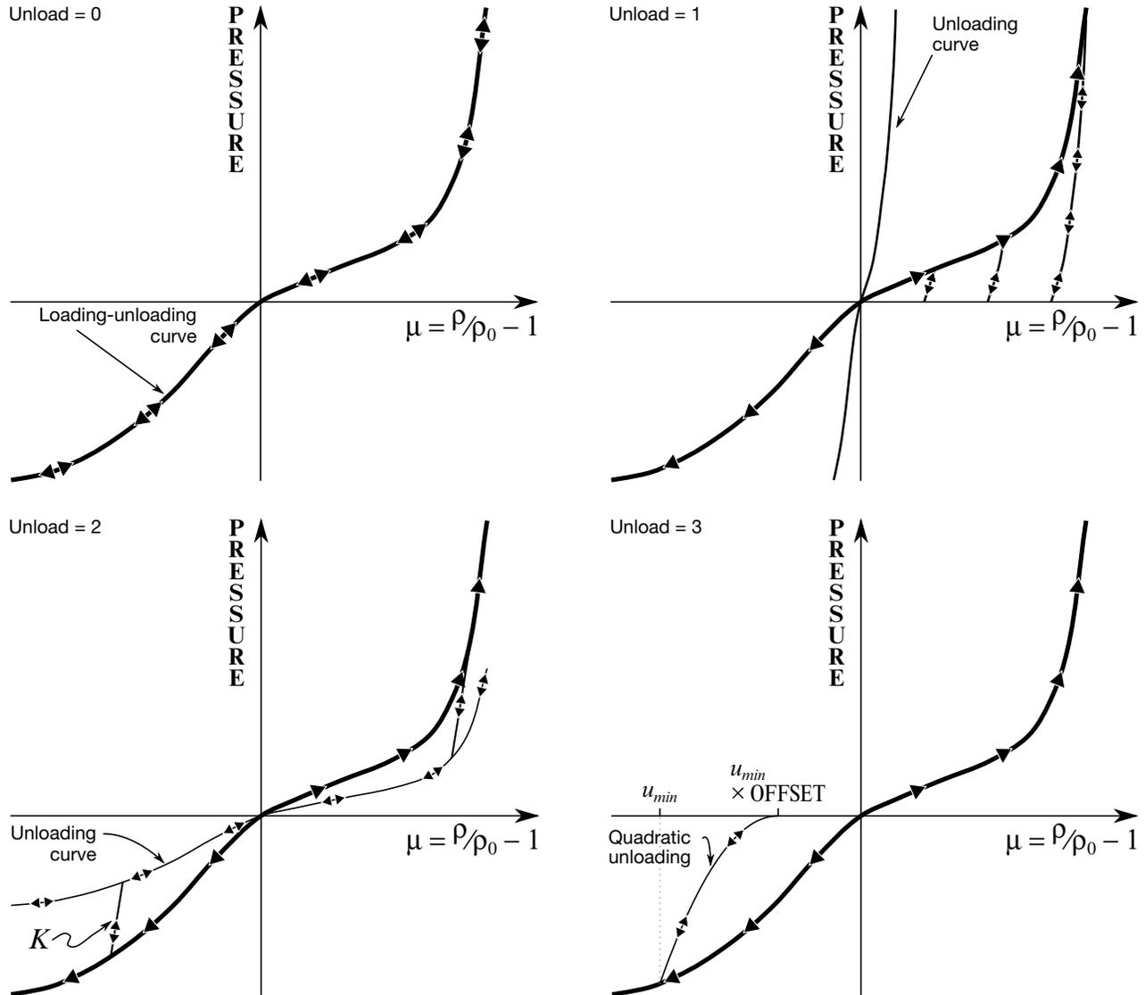
Figure EOS15-1. Load and unloading behavior.
