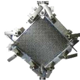
Shear: direct characterization using picture frame test
