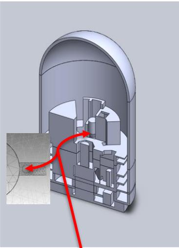
The failure locations are assumed on the pressurized tube surface
