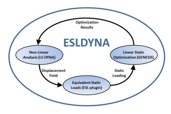
Multiple loading conditions from the nonlinear analysis can be simultaneously considered for the optimization. Each loading condition would be applied as separate loadcases on the linear structural model. ESLDYNA facilitates simultaneously running multiple LS-DYNA analyses to reduce overall design time. Most of the optimization features that are available in GENESIS can be used in ESLDYNA.
