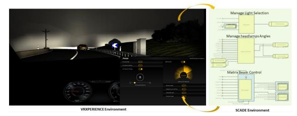
Example of a SCADE and VRXPERIENCE simulation loop for intelligent headlight control
