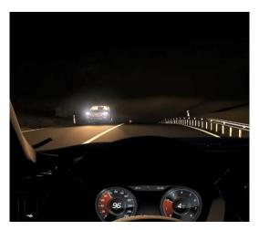
In this demo created by Ansys, a smart headlamp design can be dynamically tested to avoid glare as other cars approach.
