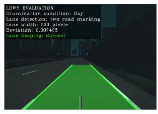
Ansys VRXPERIENCE includes a raw camera sensor model that validates the headlamp system's detection and decision algorithm at the model (MIL), software (SIL) or hardware (HIL) level.
